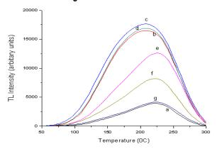
Figure 1. TL glow curve of NaCl (pure) and NaCl:Dy<sup>3+</sup> (0.05-0.5 mol%).exposed to gamma-dose = 0.50 kGy. (a)NaCl (pure), (b)NaCl:Dy<sup>3+</sup> (0.05 mol%), (c)NaCl:Dy<sup>3+</sup> (0.1 mol%), (d)NaCl:Dy<sup>3+</sup> (0.2 mol%), (e)NaCl:Dy<sup>3+</sup> (0.3 mol%), (f)NaCl:Dy<sup>3+</sup> (0.4 mol%), and (g)NaCl:Dy<sup>3+</sup> (0.5 mol%).
