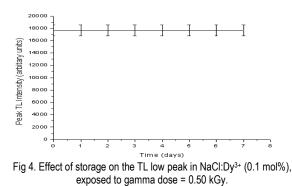
Figure 4 shows the effect of storage in dark at room temperature on the peak TL intensity in the NaCl:Dy<sup>3+</sup> (0.1 mol%) sample. From this graph it is seen that the TL peak intensity of all the samples are quite stable since there is not much fading of intensities as the loss of colouration is less in darkness [7].
