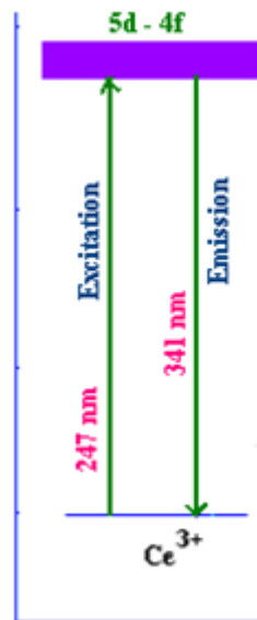
Fig 6. Schematic energy level diagram of \text{Ce}^{3+} in \text{Na}_{21}\text{Mg}(\text{SO}_4)_{10}\text{Cl}_3:\text{Ce}
