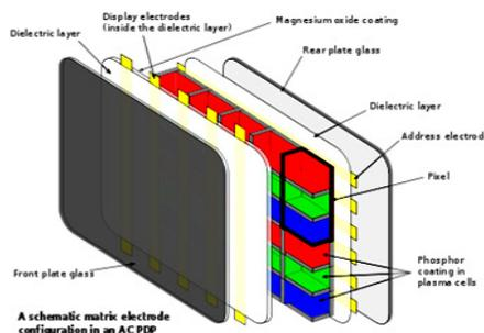
Fig 2. Composition of plasma display Panel.
