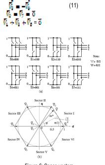
Figure 6: Space vectors. (a) Eight switching states. (b) Voltage vector space.
