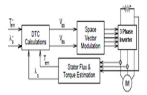
Figure 2: DTC using Space Vector Modulation Block Diagram
