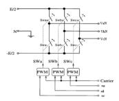
Figure 5: Three phase PWM Inverter
