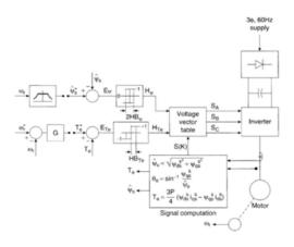
Figure 3: Direct torque and flux control block diagram
