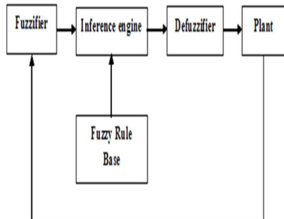
Since the FL controller processes user-defined rules governing the target control system, it can be modified and tweaked easily to improve or drastically alter system performance. New sensors can easily be incorporated into the system simply by generating appropriate governing rules.
