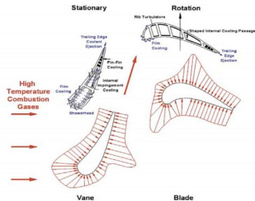
Fig. 1. Cross-Sectional View and Heat Flux Distribution of a Cooled Vane and Blade
