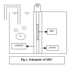
Air-saturated tap water was fed into the cathode compartment
