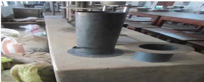
Fig 5. Sand replacement apparatus with calibrating cylinder
