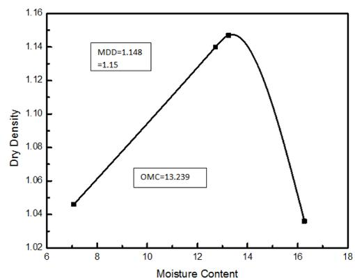
Fig 7. Diagram of maximum dry density & optimum moisture content
