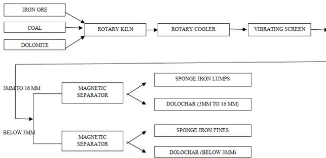
Fig 1. Schematic diagram of sponge iron production
