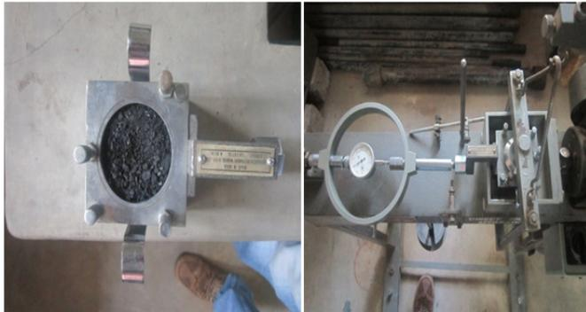
Fig 8 (a). Direct shear box
