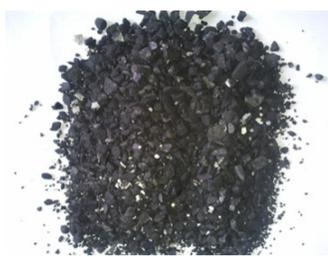
Fig 2 (a). Sample passed in 4.75mm IS sieve
