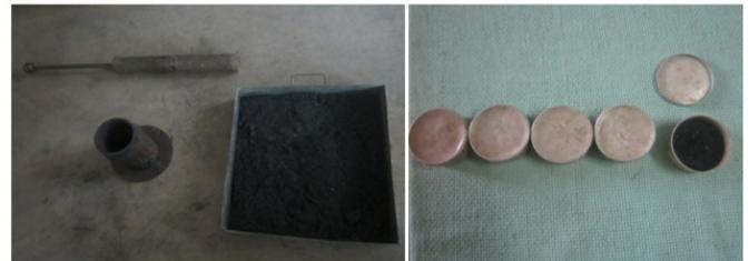
Fig 6 (a). Standard proctor mould, rammer & sample
