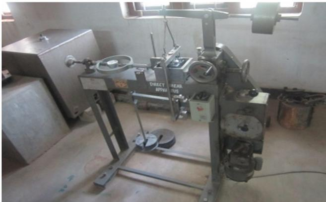
Fig 8 (c). Total arrangement of direct shear machine with loading pad
