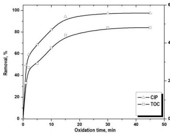
Fig 2. CIP and TOC removal with reaction time. Experimental conditions:  $[CIP]_0=15\text{mg/L}$ ,  $[Fe^{2+}/H_2O_2]_0 = 0.125 \text{ mM}$ ,  $\text{pH} = 3.5$ ,  $\text{UV} = 9\text{W}$  and  $\text{temperature} = 25^\circ\text{C}$ .
