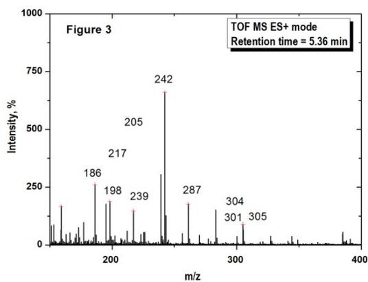
Fig 3. Mass spectra of CIP degradation recorded at 10 min of UV illumination. Experimental conditions:  $[CIP]_0=15\text{mg/L}$ ,  $[Fe^{2+}/H_2O_2]_0 = 0.125 \text{ mM}$ ,  $\text{pH} = 3.5$ ,  $\text{UV} = 9 \text{ W}$  and  $\text{temperature} = 25^\circ\text{C}$ .
