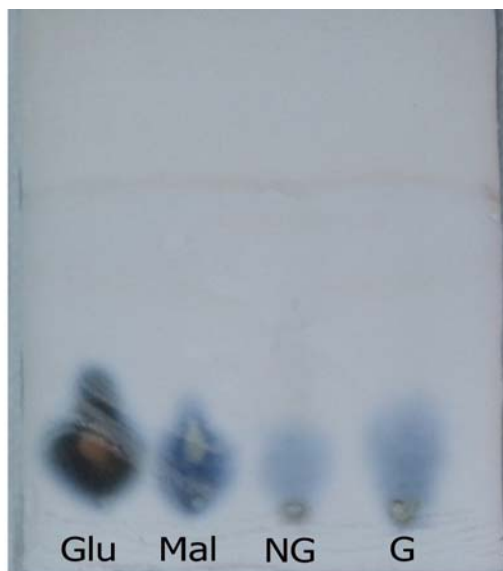
Figure 1: Thin Layer Chromatography of enzyme hydrolyzed product of non-germinated (NG) and germinated (G) seed samples. (Glu- Glucose, Mal- Maltose)
