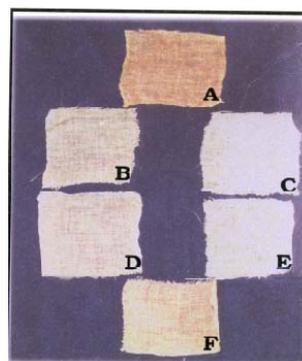
Fig7: Removal of tea stains by tannases from *A. niger* and *P. variable* at 50°C A: Washed with tap water; B: Tap water + *A. niger* tannase; C: Detergent + *A. niger* tannase; D: Tap water + *P. variable* tannase; E: Detergent + *P. variable* tannase; F: Detergent
