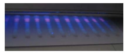
**Figure 1.** Appearance of TLC plate under 365 nm after separation of methanolic extract of *S. cumini* seeds on it. Fraction 4 and 5 are visible as red spots.
