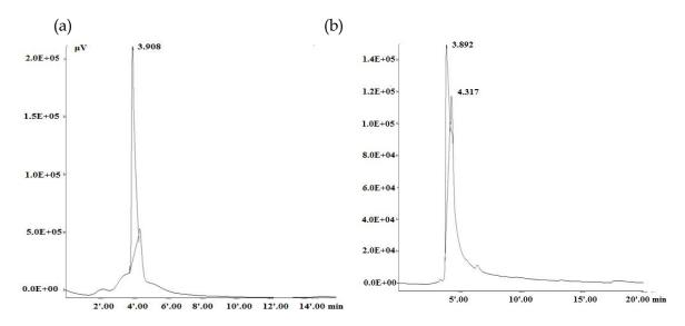
**Figure 3. Indication of gallic acid's presence in Fraction 1:** (a) Gallic acid; (b)Fraction 1; mobile phase acetonitrile:water (90:10) + acetic acid at flow rate 0.7 mL/min
