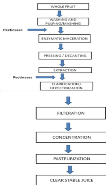
Fig.1. Pectinases at different phases of fruit juice manufacturing
