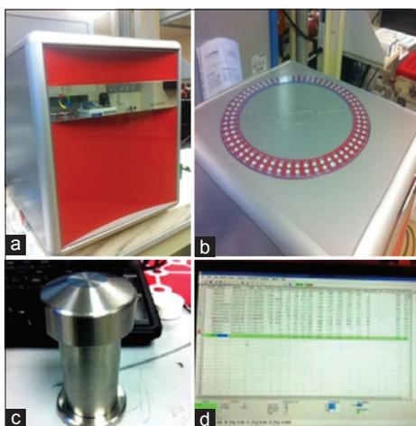
**Figure 8:** (a-d) The equipment and steps used for carbon-nitrogen-sulfur (CNS) Analyzer used to detect the CNS ratio in the three dried fruit samples of fruit *Triphala*. (a). CNS analyzer, (b) CNS carousel sample slots, (c) Aluminum Boat, (d) Data from analyses save in an Excel spreadsheet
