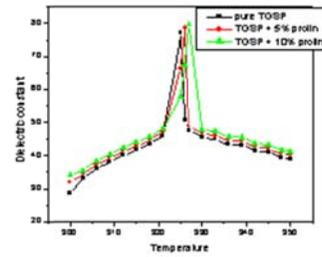
Figure 2 Variation of Dielectric constant with temperature.
