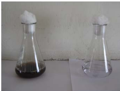
Fig .1. Image shows, 1 mM Ag no3 aqueous soln is treated with Cell biomass and D.D H2O used as a Control .Observation was taken at 48 hrs.
