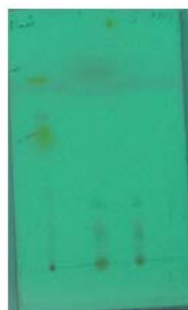
Fig.1: Spots of TLC plate containing BHT, BHA and sample seen under UV light
