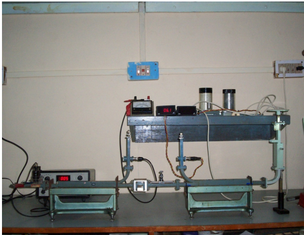
Fig 1. Microwave setup x-band at 9.85GHz frequency
