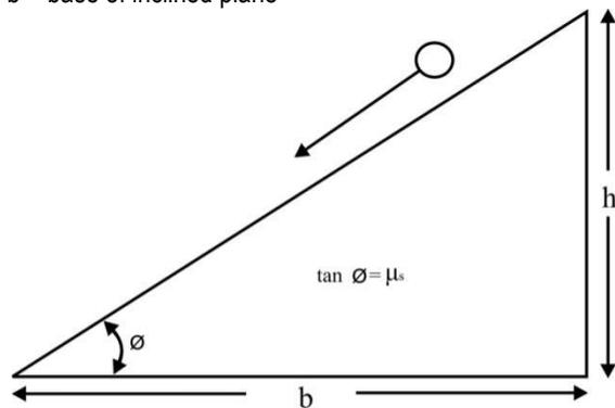
**Figure 3:** Determination of coefficient of sliding friction by inclined plane method.
