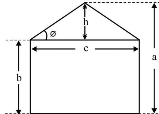
**Figure 4:** Determination of angle of repose by the cone method.
