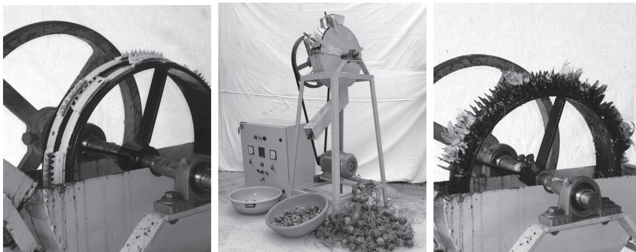
Fig. 6. Arecanut dehusker with different types of dehusking rotors
