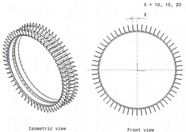
**Fig. 5. Dehusking drum with longitudinal profiled blade**
