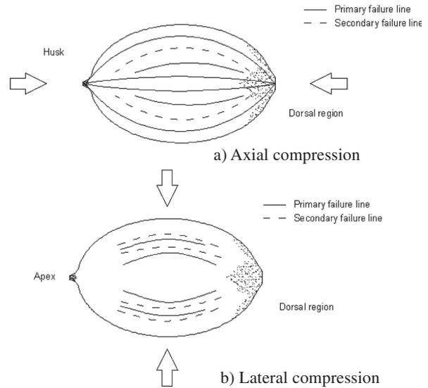
**Fig.1. Failure pattern of arecanut husk in compression**
