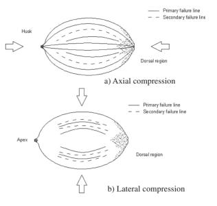
Fig.1. Failure pattern of arecanut husk in compression
