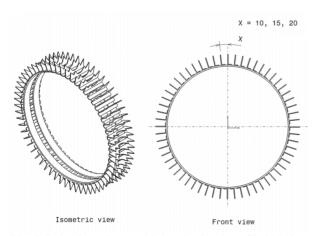
Fig. 5. Dehusking drum with longitudinal profiled blade
