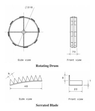
Fig. 4. Dehusking drum with saw tooth circumferential blade
