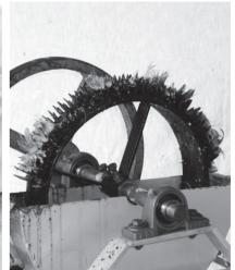
Fig. 6. Arecanut dehusker with different types of dehusking rotors
