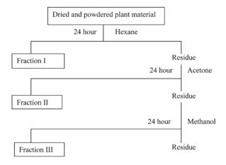
The solvents were removed under reduced pressure in a rotary evaporator to obtain semi-solid material. This material was dissolved in methanol to prepare 20 per cent stock solution from which different concentrations ranging from 1 to 4 per cent were prepared in distilled water from the stock solution.
