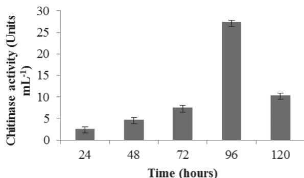
**Fig. 1. Time course of chitinase production by *P. fluorescens* in a medium supplemented with colloidal chitin as a sole carbon source. (Values represents mean of five replications ± SE)**
