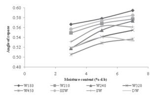
Fig. 6. Angle of repose of cashew kernels influenced by moisture content
