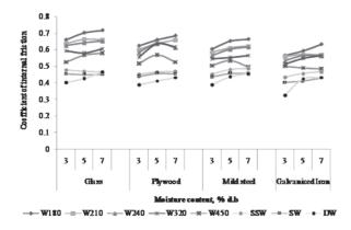
Fig. 9. Coefficient of internal friction of cashew kernels influenced by moisture content
