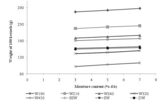
Fig. 4. Changes in weight of 100-kernels influenced by moisture content
